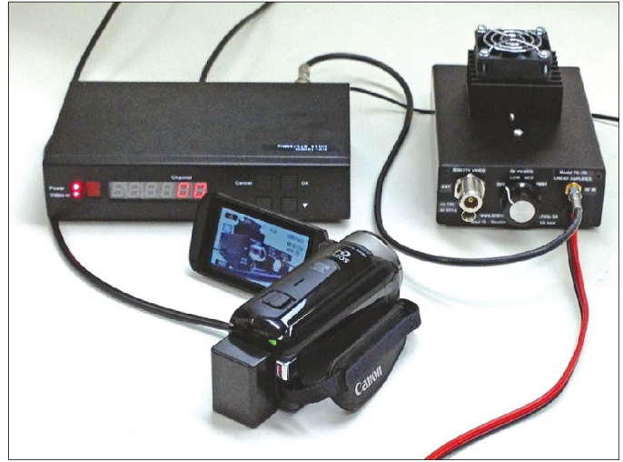
Figure 3 — Complete DVB-T TV transmitter system includes a (left) Hi-Des modulator, (right) 70 centimeter, 300 mW / 1 W / 3 W linear amplifier, and (center) high-definition camcorder.
