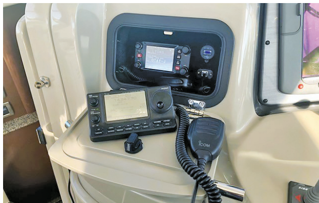
The Yaesu FTM-400 VHF and UHF radio mounted in a waterproof "glove box."
