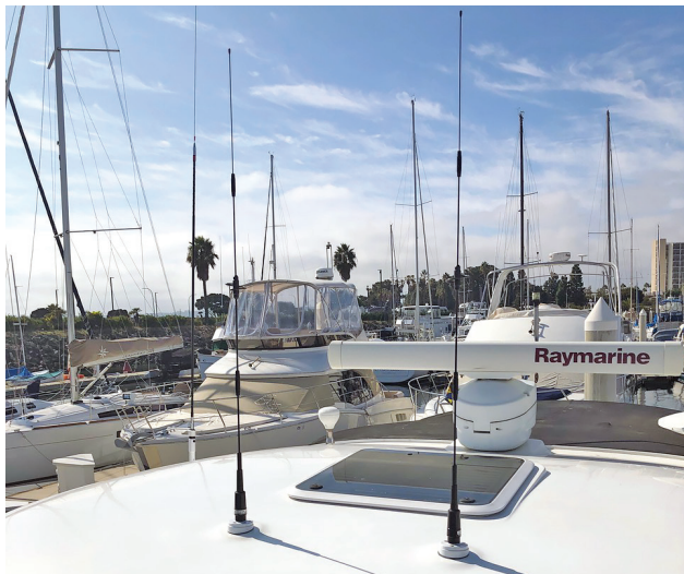
The hamstick-style antennas for VHF and UHF, custom mounted on the roof of the boat.
