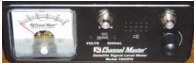
Figure 5 — CM satellite signal strength meter.
