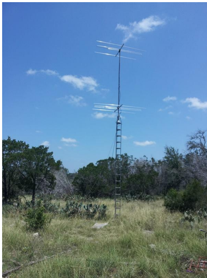
The AB5EB 3-element 6 meter OWL Yagi array. (Photo by AB5EB)
