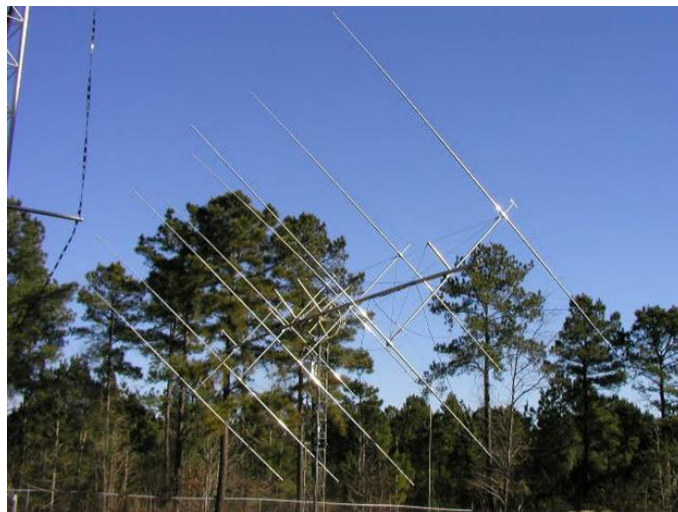
The EME array at K5QE is an array of 8 Yagis with 18 elements each (8x18) with custom elements for EME. The cross boom is 60 feet. (Photo by K5QE)
