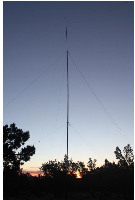
Operating portable from a cabin in Heber, Arizona at an elevation of 6,435 feet, Mike KF7ADB used a top-loaded wire vertical to work 49 states and 5 new DXCC entities. (Photo by KF7ADB)
