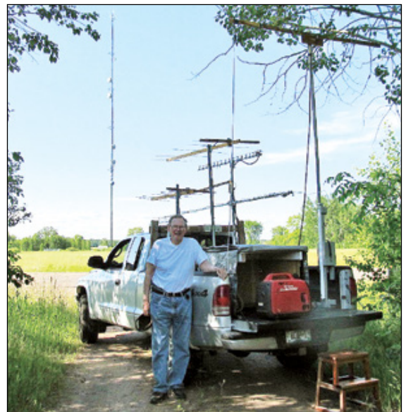
Mel Larson, KC0P/R, showing his battery-charging power source (2 kW generator) and his mobile array for his multiband operation June 2015 while roving west of Hinckley, Minnesota in grid EN36LA. [Carol Larson, N0HZO/R, photo]
