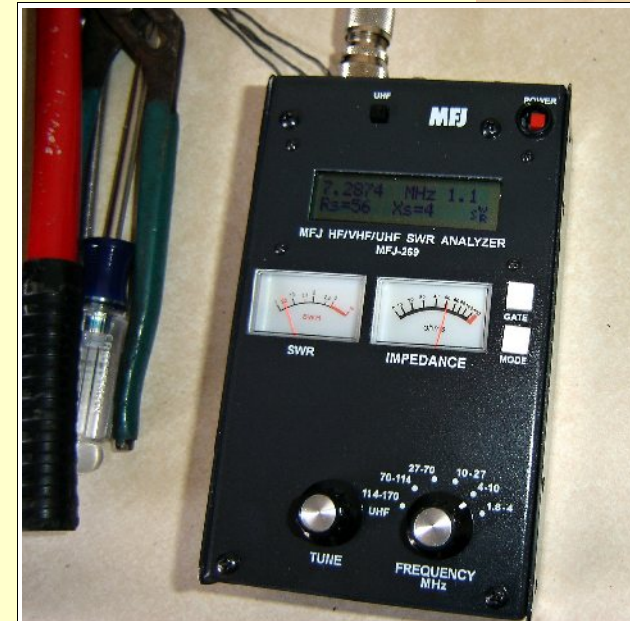
A MFJ-269 Antenna Analyzer is connected to the RG-8X coax in the building for test. It shows an excellent match at 7.28 MHz.
